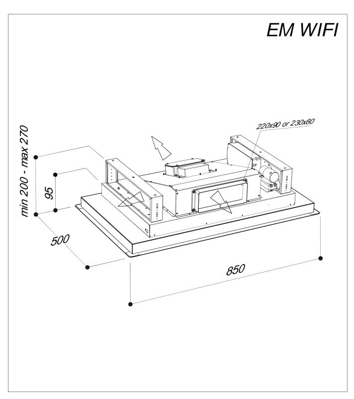
For the installation, create a false ceiling with a niche of 815mm for 465mm whose minimum height to be reached is 200mm
