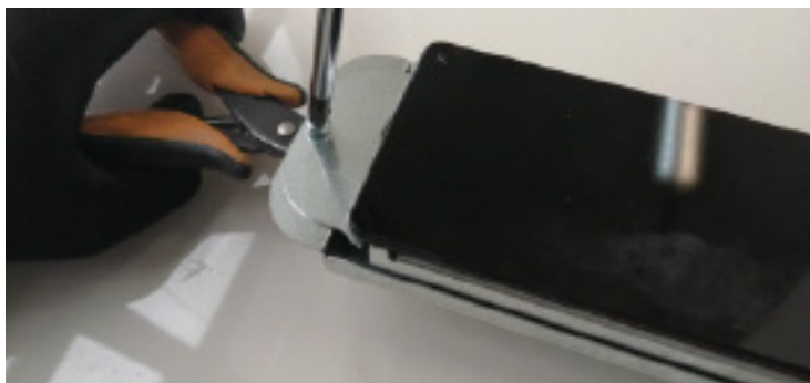
Fig.6 - Undo the two screws of the control unit
